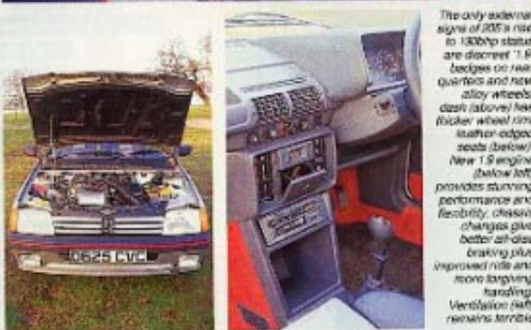
The only external signs of 205's rise to 130bhp status are discreet '1.9' badges on rear quarters and new alloy wheels; dash (above left) has thicker wheel rim, leather-edged seats (below). New 1.9 engine (below left) provides stunning performance and flexibility; chassis changes give better anti-dive braking plus improved ride and more forgiving handling. Ventilation (far right) remains torpid
